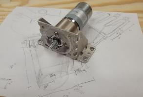
To drive the two wheels, two large motors were attached to the base chassis. These motors directly drove the two wheels, providing a large amount of torque, giving our robot the ability to maneuver effectively around the field. To help keep the remaining
