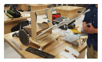
Using these materials would create a heavier design, aiding traction on the rear wheels, and creating a more rigid and stable component. Strings were then attached through I-bolts on the bottom left and right sides of the bucket, closest to the center of the robot. The string was strung through these bolts and then fastened onto the rotating shaft, allowing the driver to operate the bucket controls more easily.
