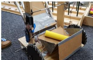
fastened to a rotating shaft, creating a pulley-like mechanism that pulls on one side of the bucket, causing the contents to fall out the other side. After prototyping our initial designs, our team created the official bucket using thin plywood in combination with cardboard.
