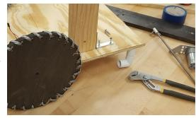
plywood level with the wheels, PVC skids were created, heating the PVC piping, and bending it to the proper position. These skids would help the robot further maneuver around the field, without limiting its ability to move. Our first skid designs consisted of an elbow piece that rested
